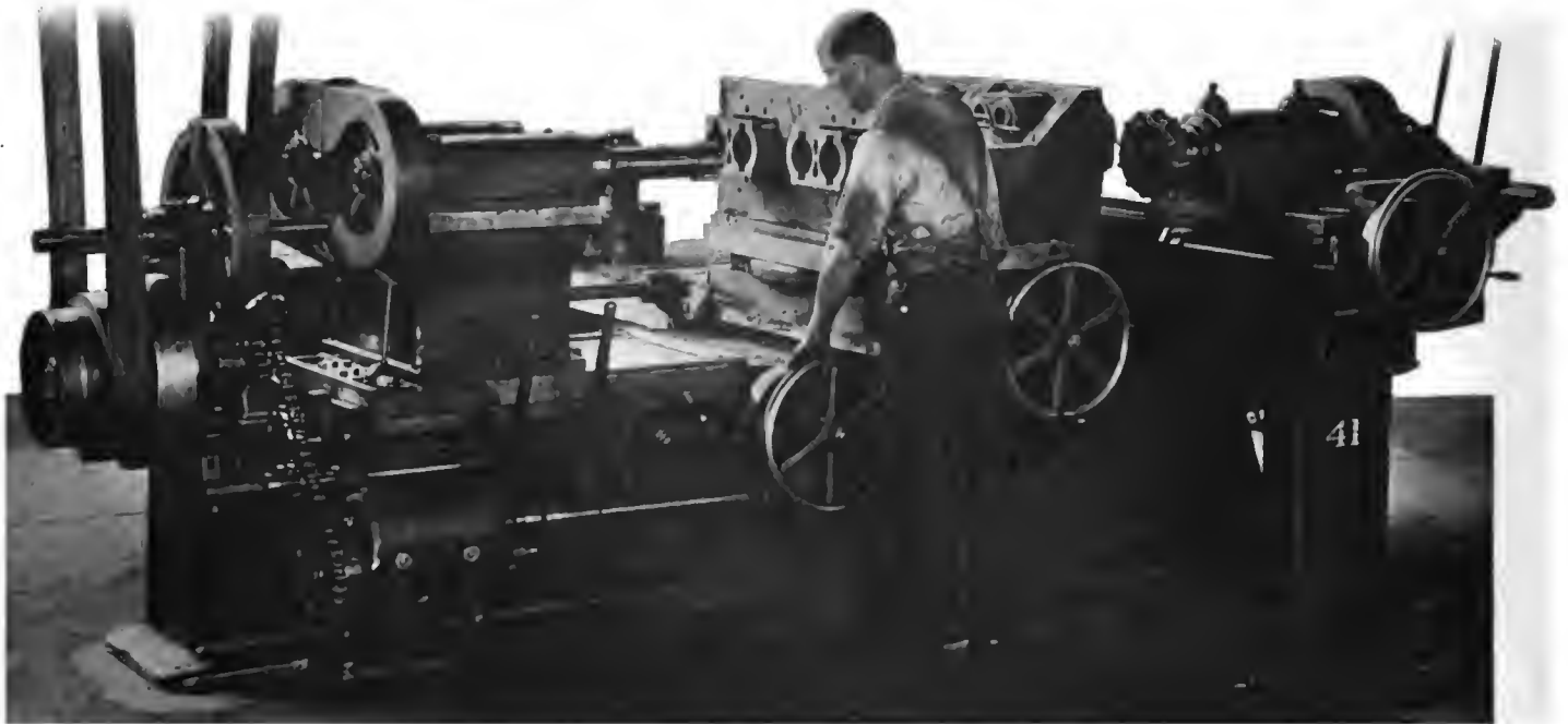
Boring machine used in the factory of the Haynes Automobile Co., Kokomo, Ind. It requires only one man to operate it
